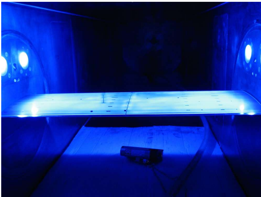
Figure 22: Illuminated TSP-model in the KRG, upstream view on the model's trailing edge
