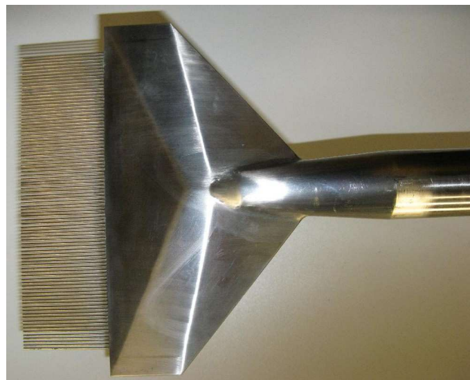
Figure 13: Wake rake with 87 pitot probes
